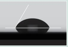
Contact angle of Oranwash L (hydrocompatible)
