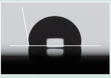
Contact angle of another well-known condensation silicone (hydrophobic)
